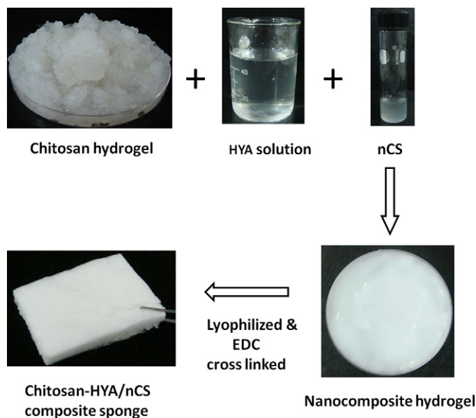
Fig. 2. Fabrication of chitosan–HYA/nCS composite sponge.
